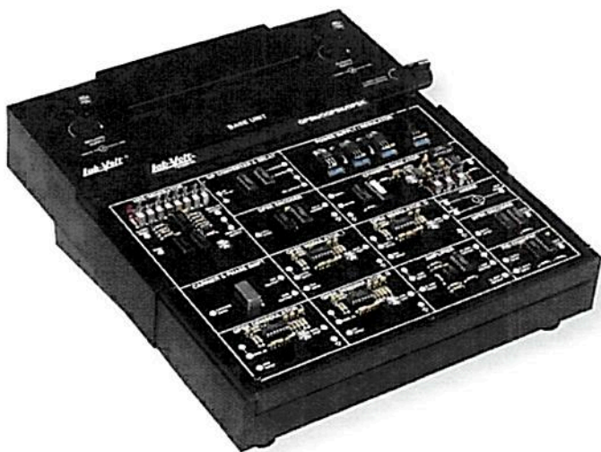
FACET boards slip easily into the base unit by means of zero-insertion force (ZIF) connectors.
